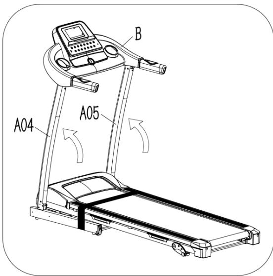
Lift the console (B) and the left and right upright tubes (A04, A05) in the direction of the arrow.
