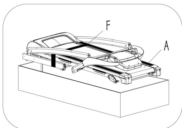
Open the box and remove the contents. Place the main frame (A) on a flat surface, make sure you have a work surface that is clean and has enough space. Do not cut the packing tape (F) before completing the assembly.
