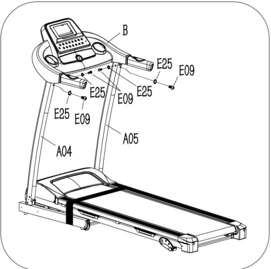
Using a 5# hex key (B08) and M8\*15 screw (E09) and lock washer (E25), lock the bracket (B) to the left and right upright tubes (A04, A05).
