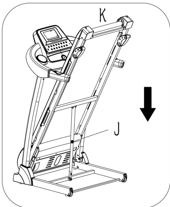
Hold the place K with your hand, press the frame lightly, then push the place J, and the base frame will automatically lower.
