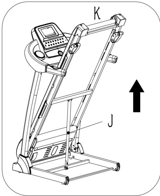
Support K with your hand, then pull up in the direction of the arrow until you hear the CYLINDER (J) lock into the round tube.
