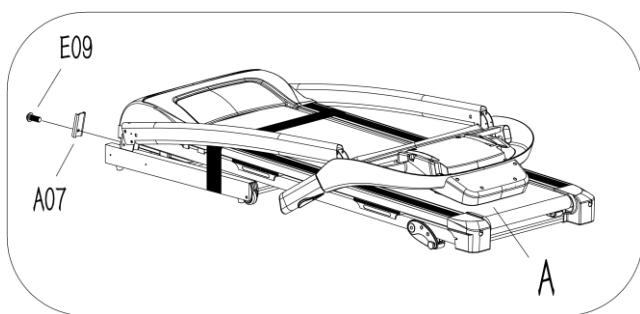
Loosen the screw (E09) on the main frame (A) using a #5 Allen key (B08) and remove the safety block (A07).
