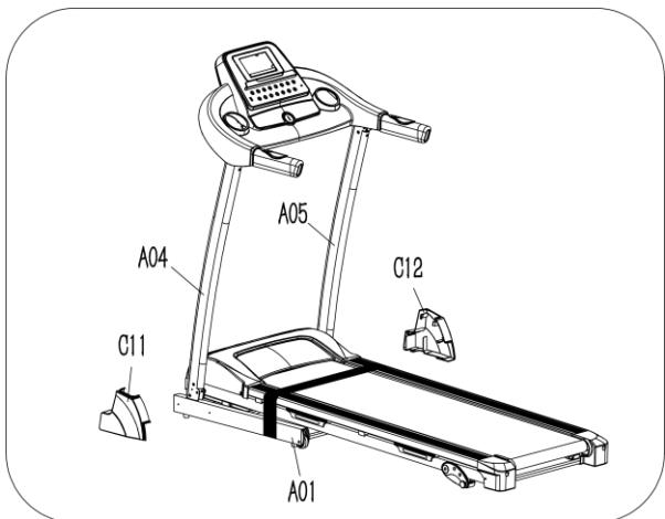
Slide the left and right tube covers (C11, C12) onto the base frame (A01), and the left and right upright tubes (A04, A05).
