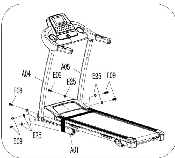
Using a 5# hex key (B08) and M8\*15 screw (E09) and lock washer (E25), lock the left and right upright tubes (A04, A05) to the main frame (A01).
