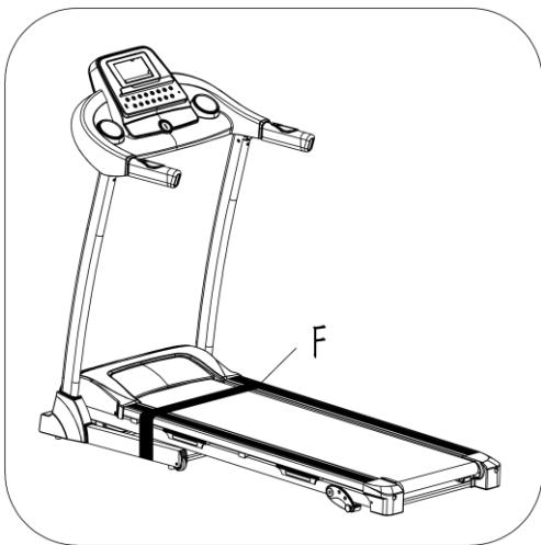
Cut the packing tape (F) after completing the assembly of the treadmill.
