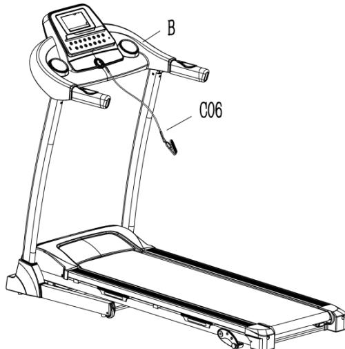
1. Before running, insert the security key (C06) into the magnetic area of the console (B) and attach the security key to your clothing (C06).
